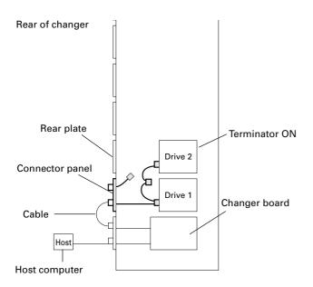
Install 6 internal drives within the changer in a daisy-chain configuration and connect the drives to the changer. (Additional cable for 4 drives will be needed.)
